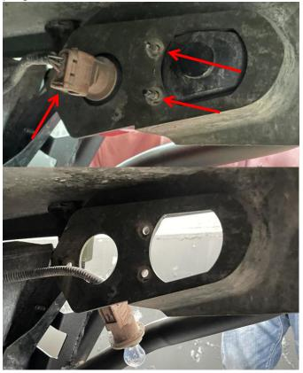
3. Before installing the new taillights, first install the wiring harness in the accessories package on the taillights; screw on the lamp head of the original car, then connect with the taillight wiring harness of the original vehicle, and finally fix the taillights in the original way.
