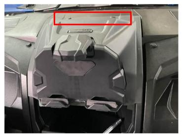
3. Open the cover of the device holder, drill two holes in the marked place with an 8MM drill bit, and then press the nylon buckles, as shown in the picture:
