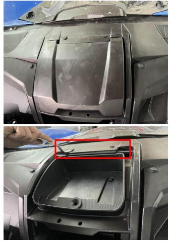
2. There is a circle of double-sided adhesive at the bottom of the device holder, tear off the release paper on the adhesive, attach the device holder to the box body, and press it slightly to make them fit better. Then press back the nylon buckles.
