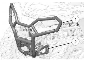
3. Install the two fasteners 3 from the front side of the front bumper into the front bumper support bracket and install the nuts 6 on the backside. Note:Do not tighten fasteners at this time.
