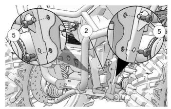
5.Torque all fasteners to specification. **Notice:** As you begin to torque the fasteners you may need to shift your bumper into place to align with the body. Then tighten all hardware.
