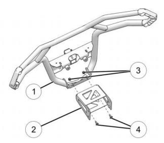
2. Install the front bumper 1 / front bumper mounting bracket 2 as an assembly and align mounting holes.
