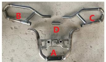
1. Fix part B and part C to part A with M8\*50 screws and nuts. As shown in picture:
