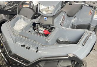
2. Move the storage rack and mounting plate from the original platform to the new platform. As shown in picture:
