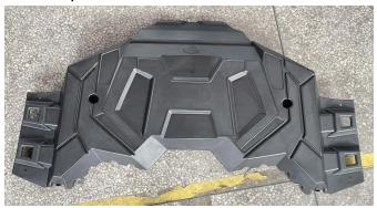
1. Open the original storage platform, remove the screws of the limit ropes inside, pry out the latches that fixed platform, and remove the platform of original vehicle. As shown in picture:
