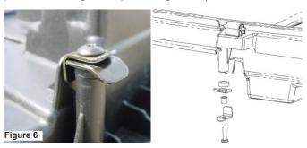
7. Install the box assembly in the opposite manner you removed the front rack by holding the rear of the box about 4 inches higher than the front. Position the front box latches in line with the rack support and slide the rack forward until the latches catch and you can not move any further forward.
