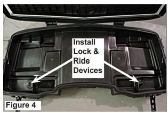
5. Assemble the two long Lock & Ride anchors (included with the front box assembly) through the base of the box per the instructions included with the Lock & Ride anchor kits. There is no self adjusting required for these Lock & Ride devices.
