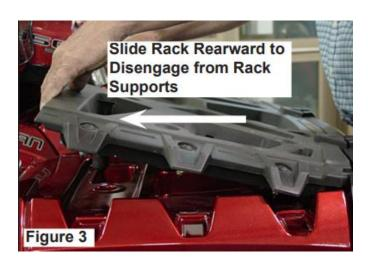
4. Remove the rack from the ATV and set aside.
