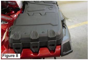
9. Verify that the box is properly installed. NOTE: The front of the box must be secure in the front rack support, check this by trying to lift up on the front of the box. If the box comes loose, repeat the process starting from Step 6.
