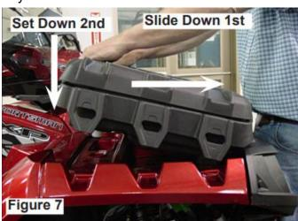
8. Lower the rear of the box and make sure it fits flat on the front of the vehicle.
