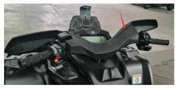
3. Secure the handguards to the handlebars with the riding clamps.
