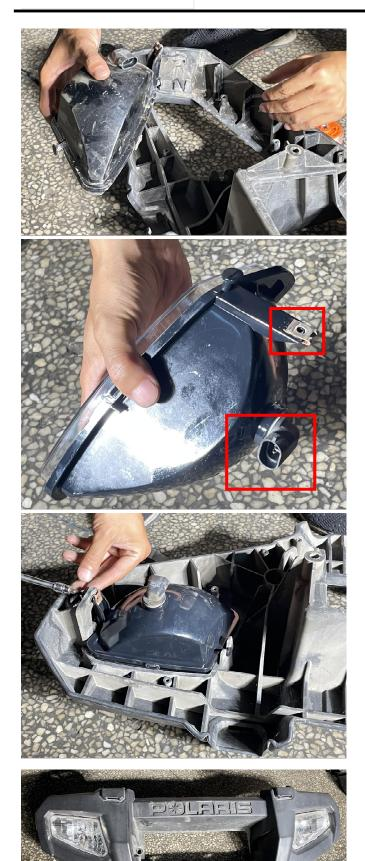
3. Put the front bar and other accessories back on the original vehicle (connect the wiring harness plug-ins of headlights before fixing). As shown in picture:
