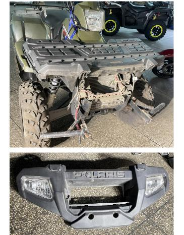
2. Remove the original headlights on the front bar, move the steel clip and bulb on the original headlight to the new headlight, and then install it back on the front bar and fix it with screws. (The headlight on other side is installed in the same way). As shown in picture:
