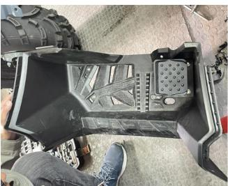
4. Install the foot pedestal on the other side as Step 1-3. Finally, the pedal and other parts removed can be installed back to the original vehicle. As shown in picture:
