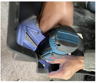
3. Place the foot pedestal on the pedal again and secure it with the screws and nuts. As shown in picture:
