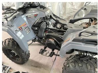
2. Place the new foot pedestal on the pedal and mark the pedal with a marker according to the positions of the fixed holes of the product. Then remove the product and drill the mounting holes by an 8mm drill bit at the place marked. As shown in picture:
