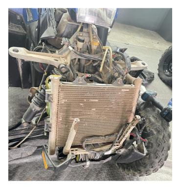
5. Remove the fan bracket of the original vehicle (remove the coolant pipe in advance), and then remove all the accessories from the original bracket and install them on the new fan bracket. As shown below:
