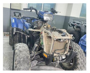
4. Unscrew the screws on the front bar frame, remove the electrical box and power supply cover on the frame, and remove the frame. As shown below:
