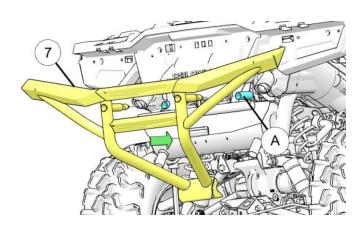
6. Tighten screws ① at this time to below specification. Final rear bumper ⑦ installation is shown below.
