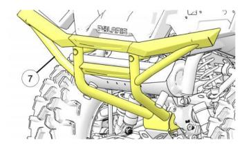
5. Slide the bumper mounting plate (a) with nuts facing down into the gap between the top of A-arm pivot and the frame (B). Insert screws (a) with lock washers (a) and flat washers (b) through the bumper (7) and vehicle frame (B) and thread into the bumper mounting plate (a). Tighten both screws (a) to below specification.
