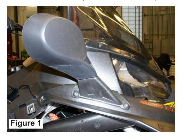
2. Use the drill and a  $\frac{1}{4}$  drill bit to drill out the center of the mounting hole.
