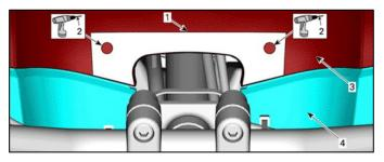
(2) Secure the gauge support into place using two plastic rivets.
