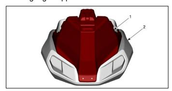
3.2 Using the smartphone support assembly as a template, drill four 5mm (3/16 in) mounting holes.
