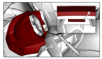
2.2 Pivot and remove the gauge support.
