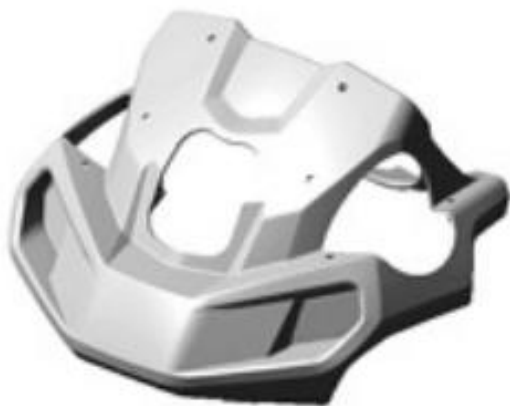
EXISTING GAUGE SUPPORT AFTER CUTOUT
