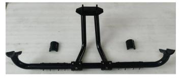
4. Fix the spare tire carrier on the rear frame with eight M8\*55 inner hexagon screws.
