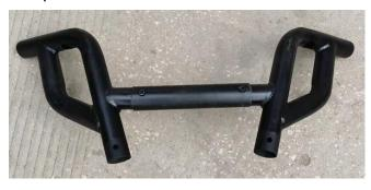
3. Assemble parts 5 and the upper part of the bumper together with four M8\*55
