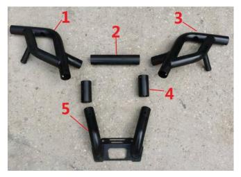
2. Assemble parts 1, 2 and 3 together with two M8\*55 hexagon socket screws and two M8 locknuts to form the upper part of the bumper.
