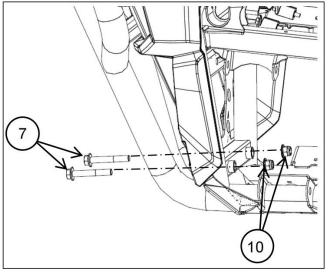
5. Screw the two remaining M8 x 16 bolts (9) through the mounting brackets (2)(3) installed previously and into the front bumper (1). Finger tighten only. (Only the left side is shown on the picture)
