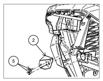
3. Place the front bumper (1) into position. Line up the holes with the mounting points of the vehicle and the brackets (2)(3) installed in the previous step.
