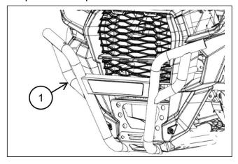
4. Install the two M10 x 70 bolts (7) and two M10 nuts (10) at the bottom of the bumper. Finger tighten only.
