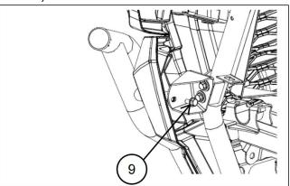
6. Tighten all the bolts. Starting with the bottom bolts.
