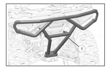
4. Install the left upper bumper fastener 3. Repeat this step to install right upper bumper fastener.
