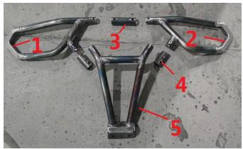
1. Assemble parts 1, 2 and 3 together with two 8\*50 hexagon socket screws and two M8 lock nuts.
