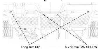
4.2 Apply upward pressure to hold storage assembly firmly against the front floor cover. Use the holes shown as a template to mark the position of 4 holes to be drilled in the floor cover.
