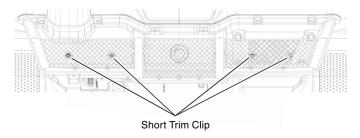
8. Install the passenger side storage net with the trim clips as shown.
