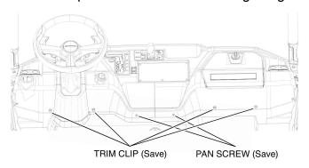
3. For vehicle after 2016 Model Year: Using the 3/8 inch drill bit, drill a hole in the front floor cover at each molded drill point as indicated below. After the holes are drilled, proceed to Step 5.
