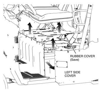
3. Slide the box bottom in from the side opening and insert the box flange through the opening under the seat.
