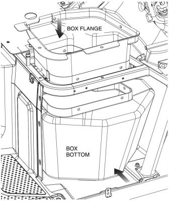
4. Align the holes between the box bottom and the box flange and connect them together with seven trim clips as shown.
