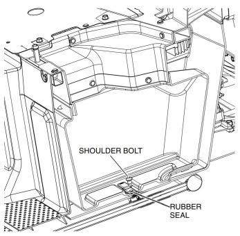
6. Referring to the Service Manual for the vehicle, re-install the seat and the left side cover using the original hardware set aside in Step 2.
