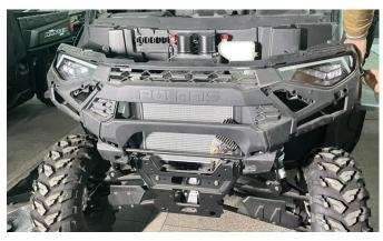
4. Remove the front bumper, then disconnect the harness plug from the headlight.
