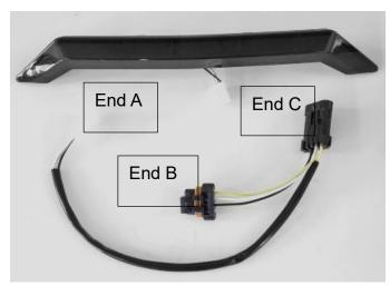
2. Remove the rear bumper of the original vehicle and disconnect the taillight wiring harness of the original vehicle. As shown in picture:
