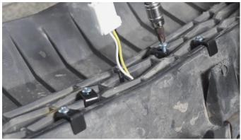
4. Take out the patch cord in the package. Connect end A with the plug-in of rear center accent light wiring harness, connect end B with the plug-in of the original vehicle taillight wiring harness, connect end C with the plug-in of the vehicle wiring harness, and finally install the rear bumper back. As shown in picture:
