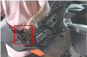
3. Pass the wiring harness of the rear accent light through the mesh grill of the rear bumper, and fix the rear accent light with a small "L" shaped bracket. As shown in picture:
