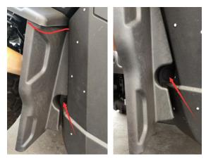
4. Refer to the location hole on the rear fender flares, and drill installation holes on the rear fender with pistol drill, then fix rear fender flares to rear fender with plastic buckles.
