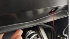
3. Refer to the hole on the fender flare, and drill a hole on the front fender with a pistol, then fix it by install the plastic buckle.
