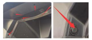
4. Align the lower fender flare with the mounting hole on the upper fender flare, and fix them together with a plastic buckle.
