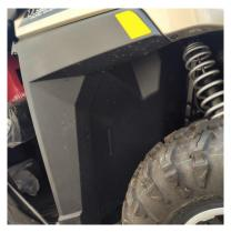
2. Align the red line on the fender flares with the outside of the fender. The big hole pointed by red arrow on the lower side is aligned with the plastic buckle that comes with the car.
