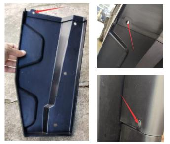
5. Align the red line edge of the lower fender flare with the outer edge of the front fender, refer to the hole on the fender flare, and drill a hole on the front fender with a pistol, then fix the fender flare with plastic buckle.
