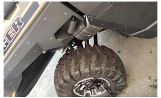
2. Align the red location line on rear fender flare with the outside edge of rear fender, then refer to the location holes, drill installation holes on rear fender with pistol drill, and fix the fender flare to rear fender with plastic buckle.
