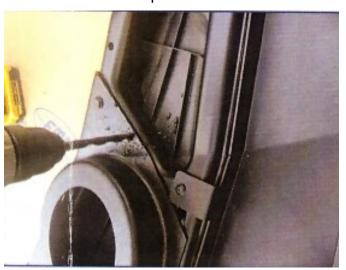
4. Using the self tapping screws and a cordless drill with a 3/8' nut driver. Run the screws through the pre-drilled holes in the pods going through the plastic and into the metal door frame. OR go straight to step 5.
