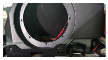
4. Use the screws in step 2 to fix the Speaker stand on the body, and then use 4x14 self-tapping screws to fix the Speaker stand on the iron bracket.
