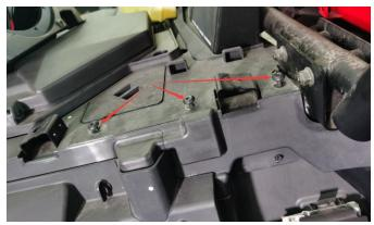
3. Use the screws in step 2 to install the iron bracket (divided into left and right) in the corresponding position. Without tightening first, mount the Speaker stand on the iron bracket. Align the holes on the Speaker stand with the holes on the car body. Then remove the Speaker stand and tighten the iron bracket.
