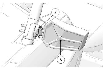
6.2 If you find it is hard to adjust the mirror, you can raise the decorative cover (8) with a slotted screwdriver, then adjusting the mirror.
