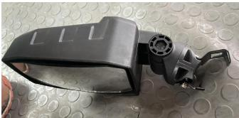
5. Snap the mounted reversing mirror bracket on the A-pillar and fix it with screws.
