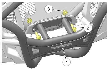
2-5. Install lower portion of bumper (1) to bumper support structure using two screws (4)
