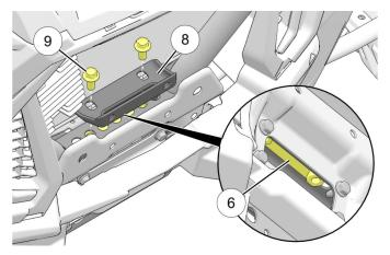
B. Loosely install upper leg of bumper support bracket (8) to suspension support structure using two each screws (9) and nuts (7).
