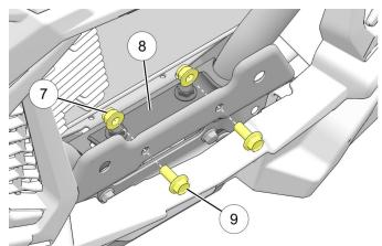
C. Torque all four screws to specification, and re-install lower front fascia using two retained screws (C) in step 2-1(B).
