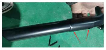
1-2. Mount part A to part D, fix them together using screws in mount hardware package, and form a complete front bumper.
