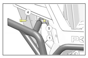
3. Place two bolts 3 through lower bumper mounts and into rear transmission bracket.
