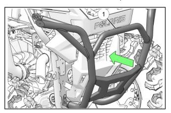
2. Place one nut 5 within each C-pillar bracket and install bumper 1 with one bolt 4 per side.
