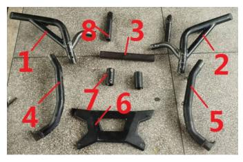
Assemble parts 1, 2 and 3 together with two M8 \* 50 hexagon socket screws, two M8 locknuts.
