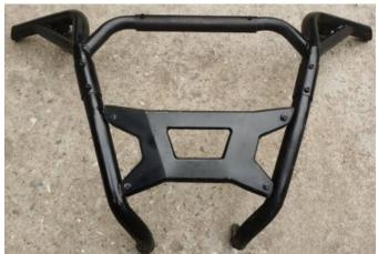
4. Assemble two parts 8 on the bar body with two M8\*50 hexagon socket screws and two M8 locknut.
