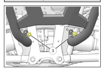
Complete lower bumper installation with two plate-nuts 2, placed on backside of rear transmission bracket. Ensure bend in plate-nuts 2 face inward and wrap around opening in rear transmission bracket.
