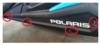
4. Fix the nerf bars rock sliders on the frame with four screws and tighten the screws.
