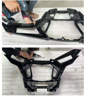
4. Remove the machine cover and front fascia
