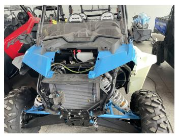
5. Install the original headlight, grille and accessories on the new front fascia according to the method when removing.
