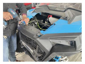
7. Connect the harness plug-in of the headlight, install the machine cover, and the installation is completed.
