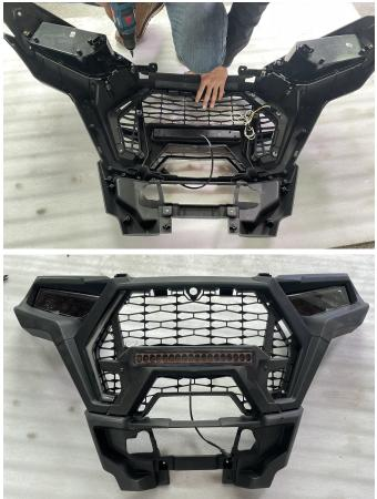
6. Install the front fascia with all accessories on the vehicle and fix it with the original vehicle screws.
