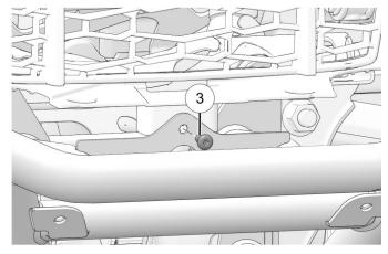
4. Install bumper plate to bumper with four plate fasteners 4.
