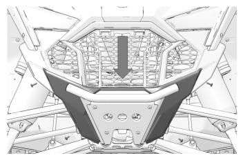
6. Reinstall top front fascia with kept fasteners (longer).
