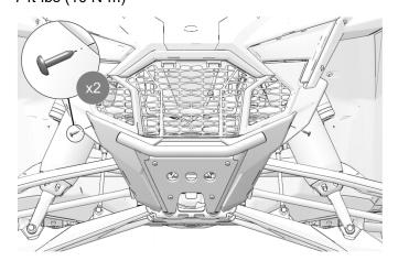
7. Reinstall bottom front fascia with kept fasteners (shorter).
