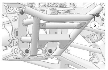
3. Secure front fascia to top of bumper with one fastener 3.
