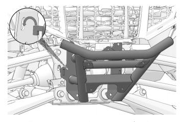
2. Install bumper to mounting plate with four bumper fasteners 5.
