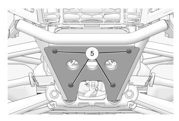
5. Reinstall front fascia panel to installed position. **Tip:** Fascia is flexible and can be carefully bent when installing over accessory bumper.
