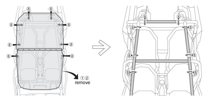
6. Reinstall the assembled roof 12 on the roll cage with two M6\*30 screws 4, two rubber washers 6, four metal washers 5, and two nuts 7.
