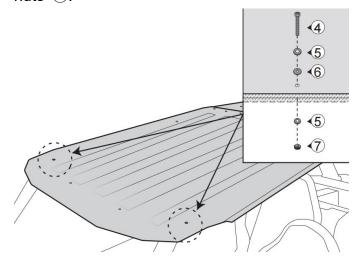
7. Use our supplied accessories to fix the assembled roof panel ①② to eight positions on the roll cage. As shown, for each mounting hole, use one M6\*30 screw ④, two metal washers ⑤, one rubber washer ⑥, one nut ⑦ and one clamp ⑧ to install.
