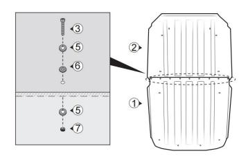
4. Place assembled roof ①② on the roll cage, loosely secure its anterior part with two original factory screws [A] and U-nuts [B] first.
