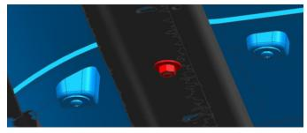
9. Fix the front end of the roof to the frame with 6x16 self-tapping screws.
