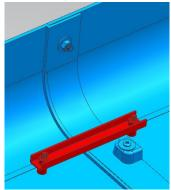
5. Unscrew the two screws in the front section of the frame and set aside. Install the roof on the frame.
