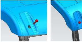
6. Use M10X25 screws to fix the back of the roof to the frame.
