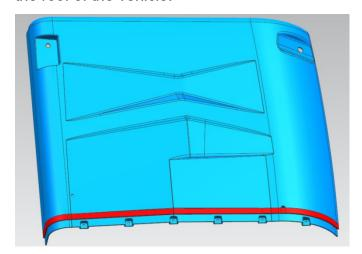
3. Use self-tapping screws 6x16 and hexagonal screws M6x20 to assemble the two halves of the roof together.
