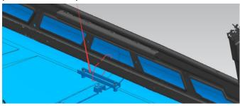
8. Use M6X30 screws to fix the front of the roof on the frame.
