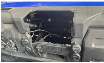
3. Fix the device holder at this position with the plastic buckles.
