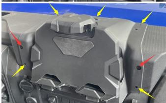
5. 8mm holes are fixed with plastic buckles, and 3.8mm holes are fixed with M5\*16 self tapping screws.
