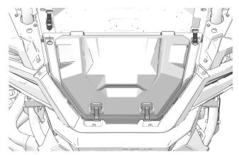
3. Lock & Ride assemblies may need adjustment. Tighten or loosen bottom nut depending on fitment.
