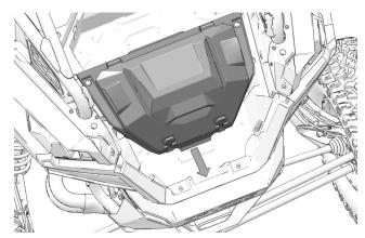
2. Place two Lock & Ride assemblies in two aligned mounting holes.
