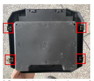
3. Remove the instrument decoration cover of the original vehicle and install the storage box. Then press hard so that the steel clips are completely stuck into the notch. As shown in picture:
