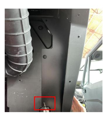
4. Place the fender on the left (main driver's seat) on the front body of the rear wheel, the holes on the fender are aligned with the holes on the car (a total of 3), and then press the nylon expansion buckle into the hole to play a fixed role.
