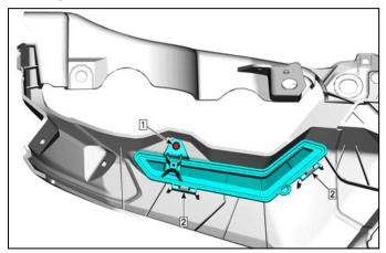
6. Install LED signature lights, secure using the previously removed screw. Tighten to specification.
