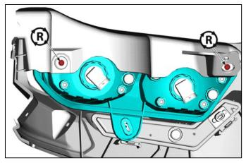
8. Reinstall the adjustment knob with washer and spring.
