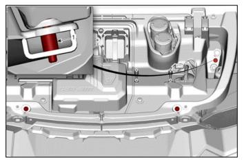
4. Disconnect headlight harness. Remove front headlight by removing the screws and adjustment knob.
