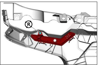
7. Reinstall headlight and secure using the previously removed screws and washers. Tighten to specification.
