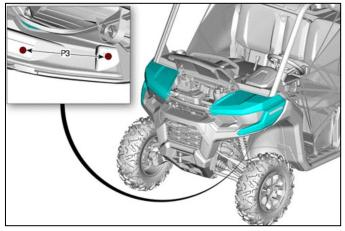
12. Secure front fascia using M6 X 20 screws. Tighten to specification. NOTICE: Ensure the spacers located underneath the service panel are still in place.
