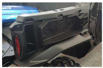
2. Remove the nuts that fixed the original lamp and take out the plug. Remove the taillight.
