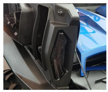
4. Install the side panels of the tail box. Installation of the taillights finished.
