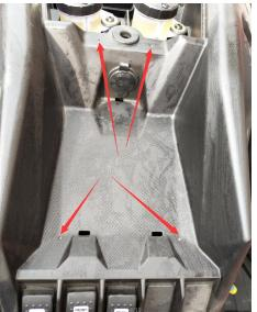
Place this holder on the instrument panel, align the 4 mounting holes on the panel with the anchor points found in step 2 & 3.
