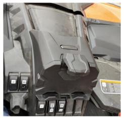
**5** Use the 5x40 self-tapping screws and flat pads in the package, and fix the electronic device holder on the instrument panel.
