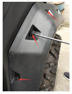
4. Refer to the holes on front fender flare, and drill installation holes on front fender by 3mm twist pistol drill. Then, fix front fender flare to vehicle by 5X40 self-tapping screws.
