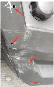
8. Insert the rubber plugs with clip to the 12.5mm installation holes.
