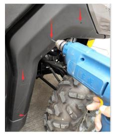
3. Fix the front fender flare to the front fender by 5X40 self-tapping screws.
