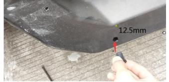
9. Fix the lower rear fender flare to vehicle by M6x25 and M6x30 screws.
