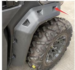
5. Drill location holes on rear fender by 3mm twist pistol drill.
