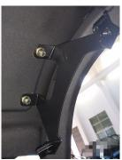
5. Install the bracket assembled in step 2 to the middle of the roof bracket. And align the hole pointed by the red arrow with the hole on the frame. Fasten with screws.
