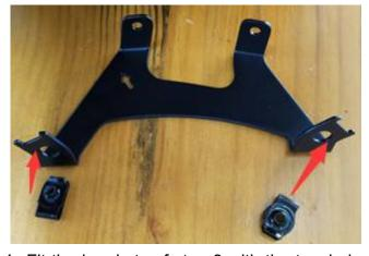
4. Fit the brackets of step 3 with the two holes on both sides of the roof bracket as shown in the figure below, and fasten them with screws.
