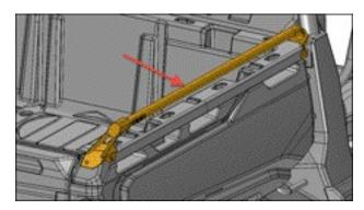
2. While firmly pressing the rail against the vehicle bed, mark the six (6) holes to be drilled with a color marker using the existing holes in the side rail as a template.
