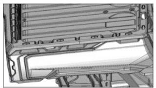
4. Punch the vehicle bed where the six(6) marks were made.
