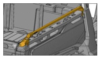
2. Screw in six Ø 5 mm self-tapping screws.
