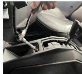
3. Find the round black waterproof plug below the accelerator pedal and remove the plug.
