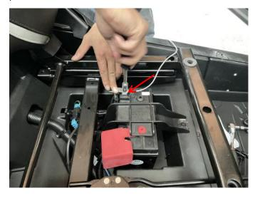
5. After connecting the negative wire, through the wire harness out from the hole under the accelerator pedal, and hide the exposed wire along the edge of
