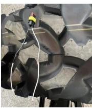
8. The connected wire harness is routed to the position of the front middle net. The excessive wire can be fixed along the line direction outside the car ,to prevent falling, as shown in the figure:
