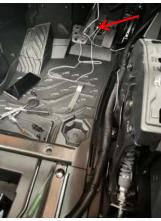
6. Find the electrical box on the left of steering wheel, take off the outer protection cover, pull up the red pin in the lower left of the electrical box, take another white wire, peel off the skin of one end, reveal the copper wire, to connect with the place where just pull up the red pin, press the red pin back after connecting, through the rest of the line out from the hole under the accelerator pedal (refer to the picture of above step): as shown in the figure
