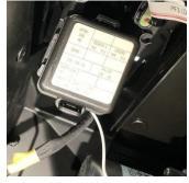
7. Unplug the connector of the wiring harness of the lamp, find the two white wires through the hole under the accelerator pedal, and connect them with the wiring harness on the lamp,the wiring harness on the battery is negative, connect the black wire, and the wiring harness on the electrical box is positive, connect the gray wire. Insulation measures should be
