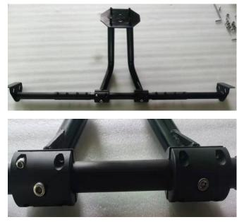
4. Fix the spare tire rack on the rear frame with four M8\*70 inner hexagon screws, four M8 flat pads and four M8 locknuts.
