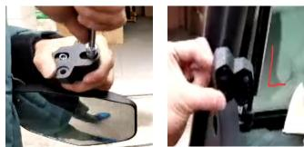
4. Put the iron holder into the vehicle frame as shown, fix the side mirror together with the iron holder by the bolts from the outside.
