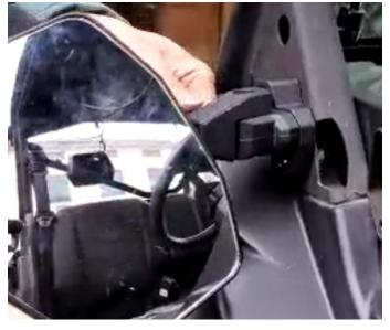
6. Adjust the angle of the mirror, then tighten the three screws at the back.
