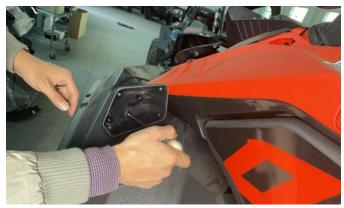
3. Fix the lens bottom bracket on the rear shell with 4 screws, and then wipe the surface of the lens bracket with the Adhesion promoter wipes in the accessories bag.
