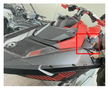
2. Fix the rear housing of the mirror with the screws in the accessories bag (the screws need to be padded).
