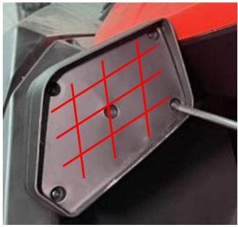
4. After the adhesive aid on the surface of the mirror holder is dry, remove the protective film on the back of the lens, paste the lens and press it hard.
