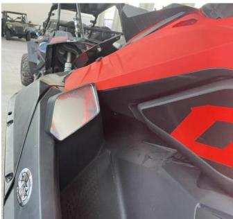
5. After installing the lens, tear off the protective film on the surface of the mirror and the installation of the mirror is completed (the mirror on the other side is completed according to the same steps).
