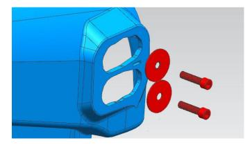
8. Install the U-nuts, spacers and screws one by one in the order shown in the figure.
