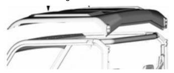
7. Install the 4 pieces of M8 large spacers and screws as shown in the figure.
