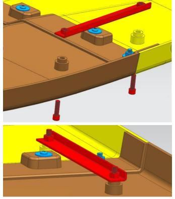
5. Bolt the front part of the roof to the frame as shown.
