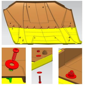
4. Install the iron brackets on both sides of the roof as shown in the figure.
