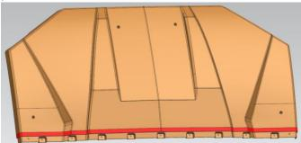
3. The front roof and the middle of the rear roof are fastened with nine 6x16 self-tapping screws. Both ends are fastened with screw nuts.
