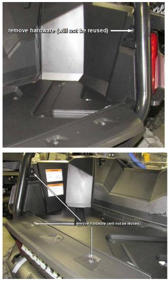
3. Install to machine with hardware as shown.
